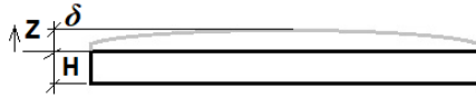
Fig. S1 Schematic illustration of a constrained thin hydrogel layer, related to STAR Methods. The initial state is assumed to be isotropically swollen from the dry state with the relevant geometrical parameters: displacement ( \delta ), material thickness ( H ).
