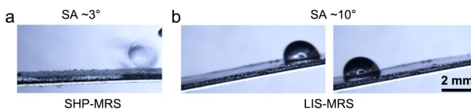
Figure S7. Sliding angle (SA) of a water droplet ( \sim 5 \mu\text{L} ): a) SHP-MRS; b) LIS-MRS. SHP-MRS exhibits superhydrophobicity with teeny adhesion. LIS-MRS coated with silicone oil exhibits excellent slippery performance.
