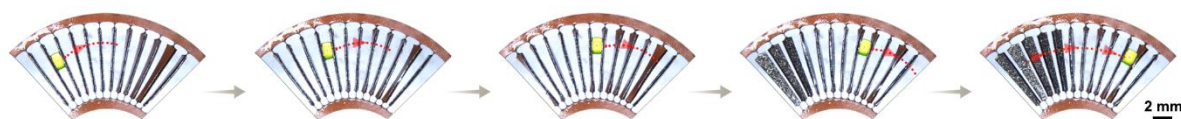
Figure S27. Droplet transport in the intervals of fan-shaped LIS-MRS. The droplet also can be transported in a particular arc path using a fan-shaped LIS-MRS, further manifesting the droplet transport ability.
