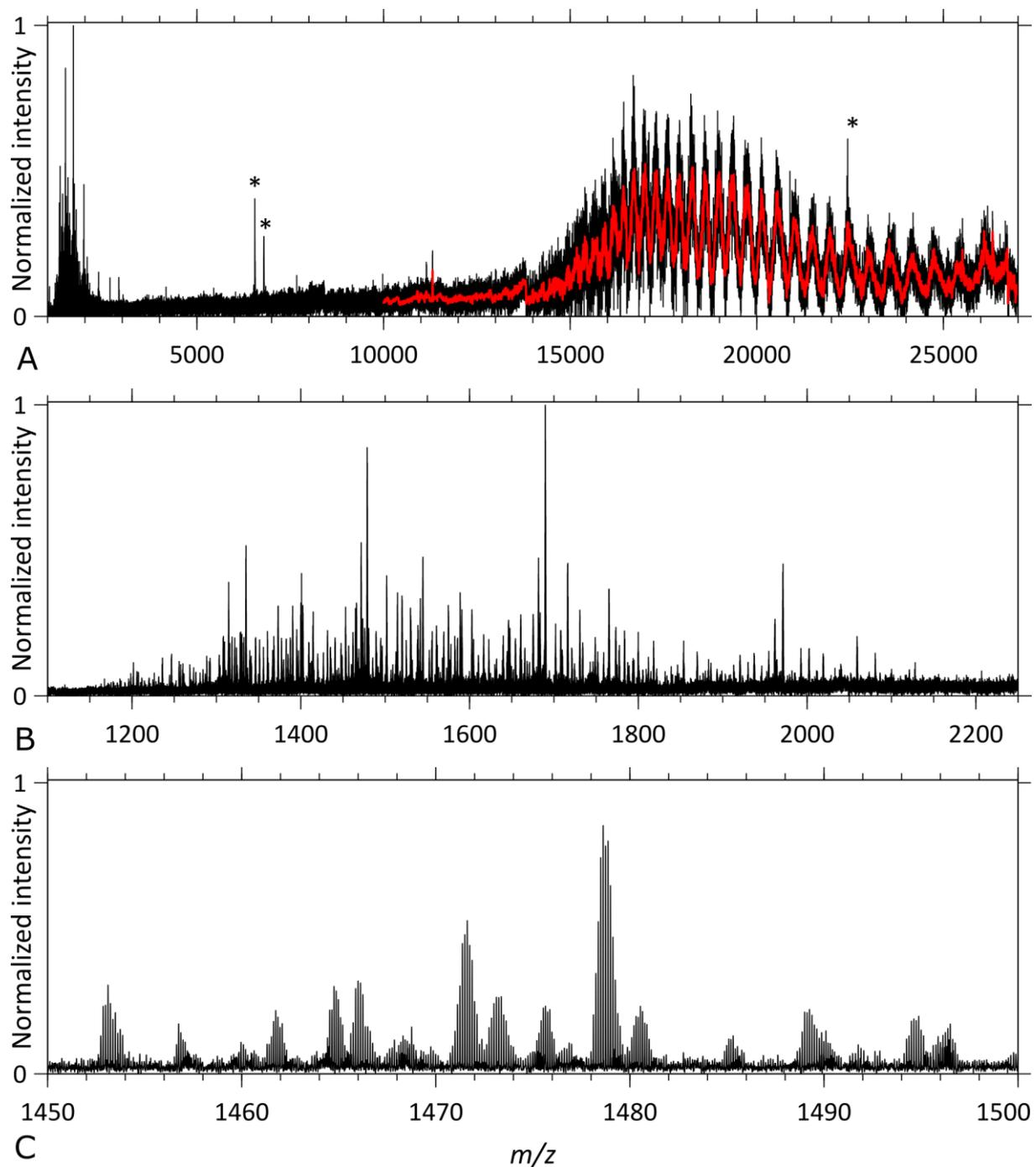
**Figure S4. Native top-down ECD MS2 spectra of the aWTA IgM assembly.** All these ECD MS2 spectra were taken with the “Analyzer CE-Inject (V) UHMR” at its default value of 3200. A) displaying the precursor ion signal at high  $m/z$ , and B) backbone fragment ions below  $m/z$  3000. C) Illustration of some of the isotopically resolved fragment ion signals.
