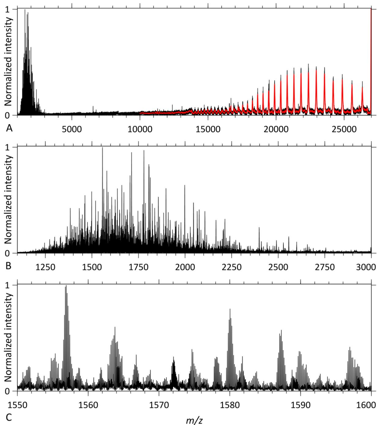
**Figure S10. Native top-down ECD MS2 spectra of the hexameric aCD52 IgG1 assembly.** All these spectra were taken with the “Analyzer CE-Inject (V) UHMR” at its default value of 3200. A) displaying the precursor ion signal at high  $m/z$ , and B) backbone fragment ions below  $m/z$  3000. C) Illustration of some of the isotopically resolved fragment ion signals.
