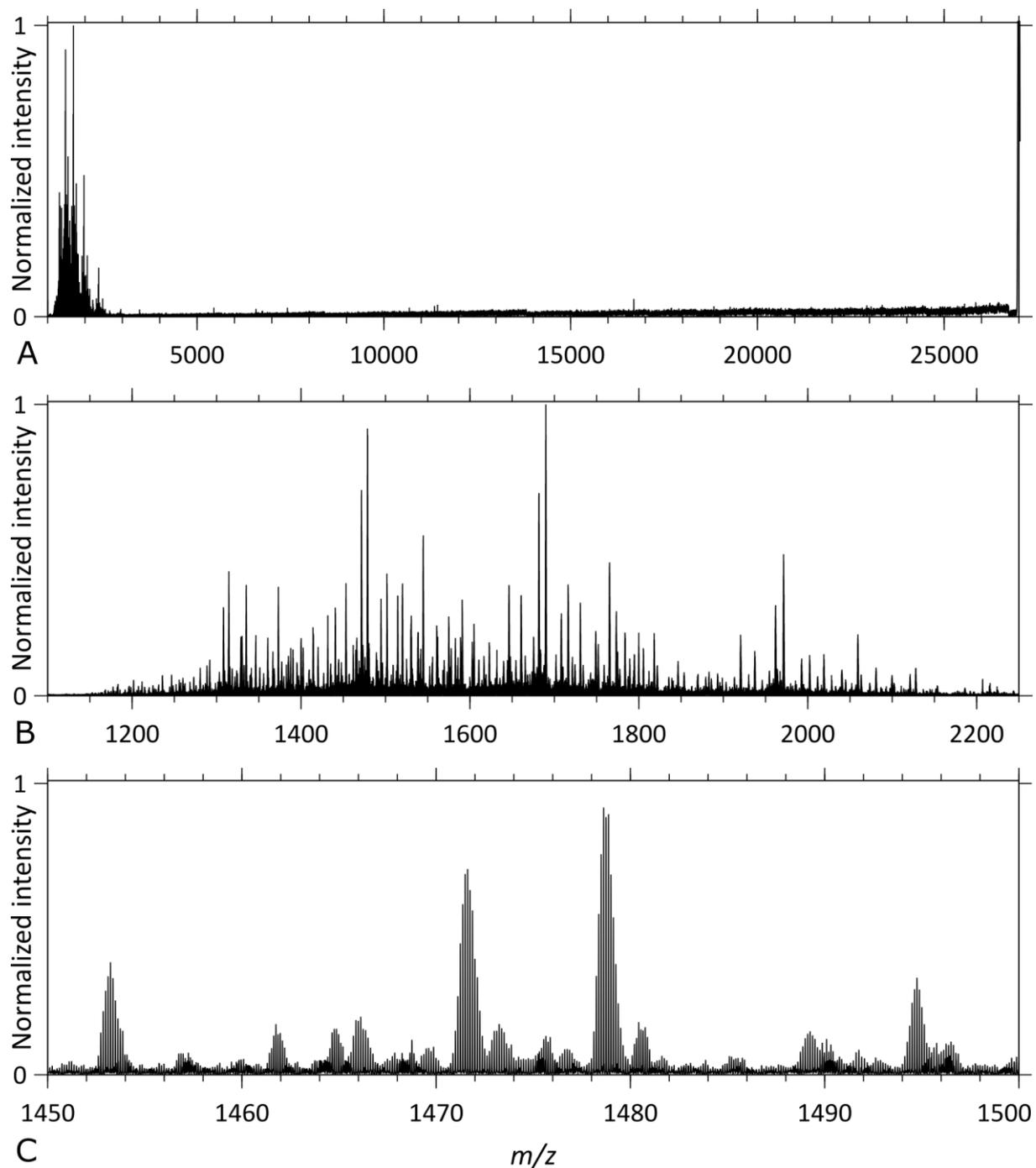
**Figure S7. Native top-down ECD MS2 spectra of the aWTA IgM assembly.** All these ECD MS2 spectra of the aWTA IgM assembly were taken with the “Analyzer CE-Inject (V) UHMR” at a value of 3700, A) displaying the precursor ion signal at high  $m/z$ , and B) backbone fragment ions below  $m/z$  3000. C) Illustration of some of the isotopically resolved fragment ion signals.
