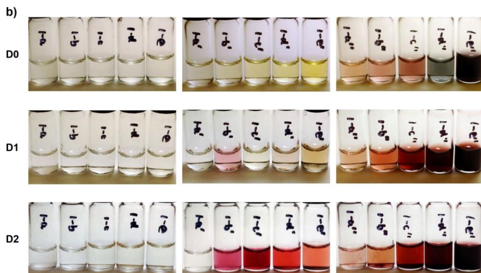
Figure S1. Growth of GS-AuNPs in solution under different conditions. The GS-AuNPs were synthesized under different gold-to-thiol (Au:GSH) ratio and pH conditions (a), where the increased Au:GSH ratio and pH value were found to increase both the reduction rates and AuNP sizes (b). In addition, the reduction of the formaldehyde 1 concentration could decrease the reduction rate. For the in situ GSH-directed AuNP growth on biological tissues, Au:GSH ratio of 1:1 and a neutral pH ( trial 1-b' ) was chosen.
