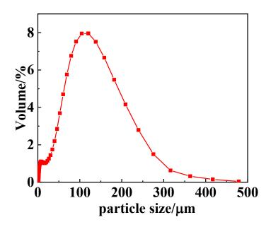
Figure S1. Particle size distribution of AL
