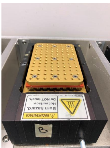
Figure S3. Representative image of a reaction block inside a heating jacket on a tumble stirrer used in high throughput experimentation.
