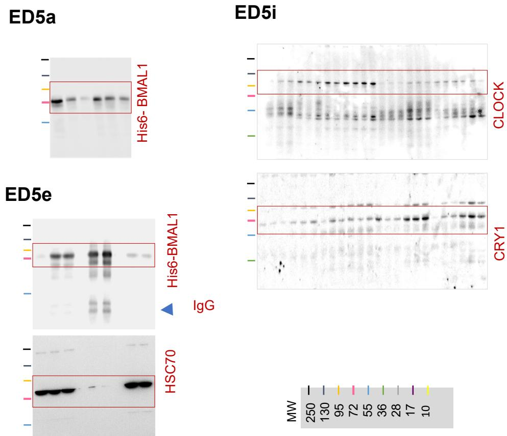
**Uncropped gels Extended Data Figure 5.** Red square indicates the section shown in the main figures. Molecular weight markers are shown on the left. \* indicates non-related band resulting from reblotting
