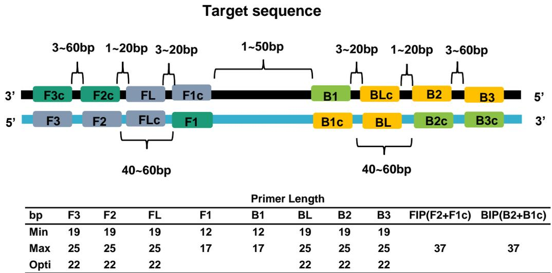
**Figure S2. Restraints on the relative position and length of the LAMP primers.**
