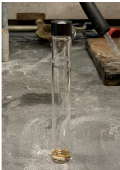
Figure S18. Reaction solution in tall 10 mL vial before heating in THF/toluene.
