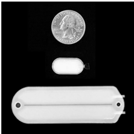
Figure 1. The two different types of units used in the present study (Upper photo) Sentinels (VC-02-20), which are smaller in size (1.5 cm x 1 cm) and have fewer cells, are explanted and examined periodically to evaluate status of the dose-finding units. For size comparison a US quarter is shown. (Lower photo) The larger dose-finding units (VC-02-300, 9 cm x 3 cm) are used to develop the procedures and to assess the safety and efficacy of various quanta of cell doses.
