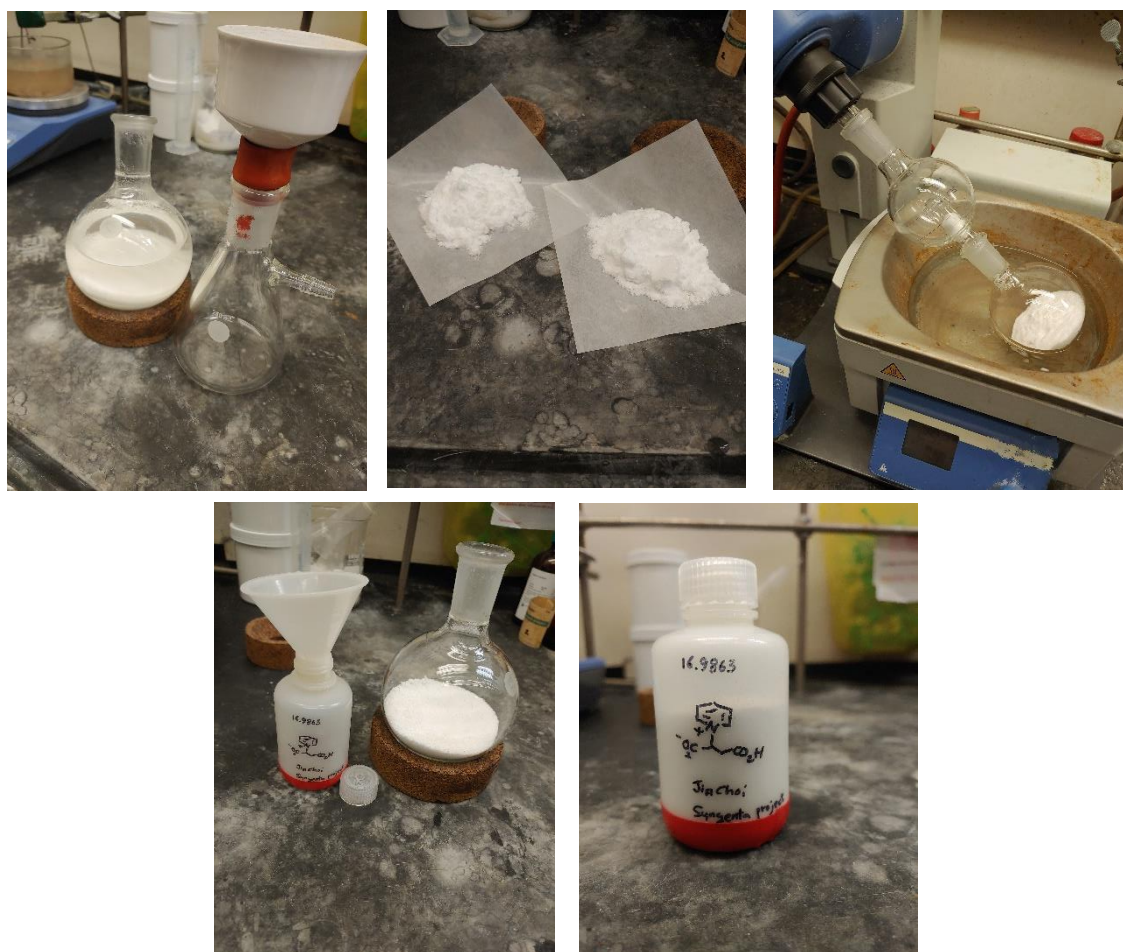
Fig. S8. Work-up procedure for the 1 st step of the synthesis of pyridinium salt 6a. Filtration of the white solid using Büchner funnel (upper left, center). The resulting solid was dried by rotary evaporator and high vacuum. (upper right), The pyridinium salt 9 was stored in 100 mL Nalgene bottle, stable in ambient temperature (bottom).
