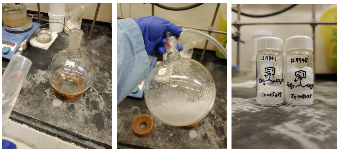
Fig. S14. Isolation of pyridinium salt 6a . Anhydrous \text{Et}_2\text{O} was added to the oil to remove the residual solvent (left), dried product obtained as a white solid (center), The resulting salt 6a was stored in 20 mL vial, stable in ambient temperature (right).
