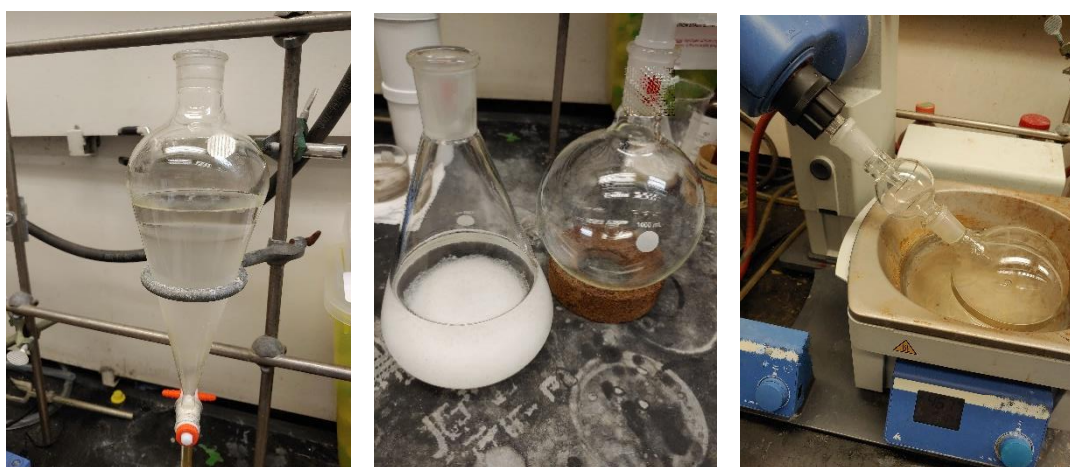
Fig. S13. Work-up procedure for to 2 nd step of pyridinium salt 6a synthesis (continued). Extraction with \text{CH}_2\text{Cl}_2 and \text{H}_2\text{O} (left), organic layers dried with \text{Na}_2\text{SO}_4 (center), filtration and evaporation of the residual solvent by rotary evaporator (right).
