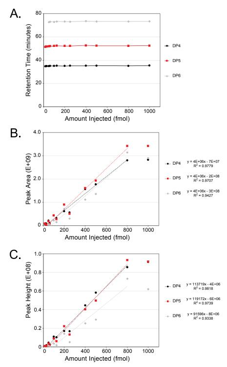
**Supplement 3. Limit of Detection.** Reduced and <sup>13</sup>C-permethylated isomalto analytical standards DP4-6 were analyzed by LC-NSI-MS at different amounts ranging from 15.625 to 1000 femtomoles injected and EICs were evaluated based on (**A**) Peak apex retention time, (**B**) Peak Area, and (**C**) Peak Height. Regression analysis in B and C was performed over the range 50-800 fmol injected.
