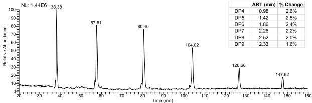
**Supplement 2. Reproducibility of standard performance.** (**A**) Reduced and <sup>13</sup>C-permethylated Dextran (isomaltooligosaccharide series, DP4 to 9) was separated using a PepMap Acclaim C18 column in 1 mM lithium acetate-containing mobile phases (45-70% B over 150 mins). Extracted ion chromatogram for each predicted mass is shown (within 10 ppm). (**B**) Rerun of Dextran after 25 days of continuously running samples.
