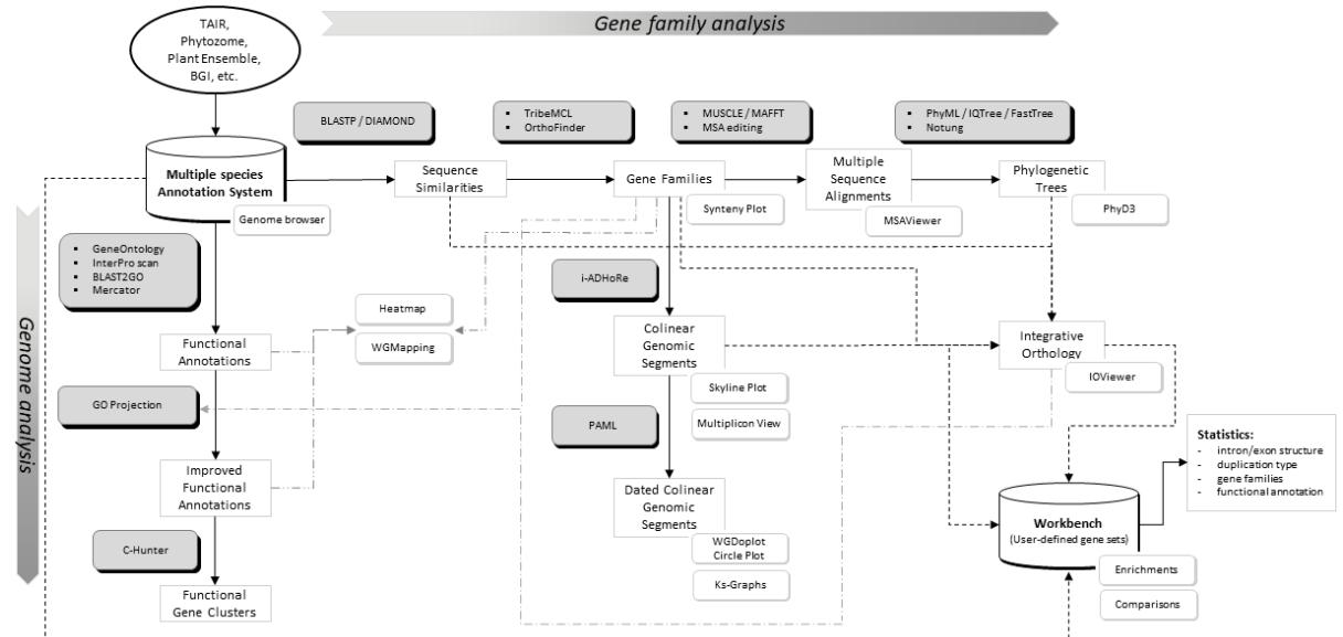
Flowchart depicting the different steps used to build the PLAZA platform. Grey boxes represent methods & tools whereas white shadowed boxes refer to website visualization tools. A detailed description of the construction steps and program settings is given below.
