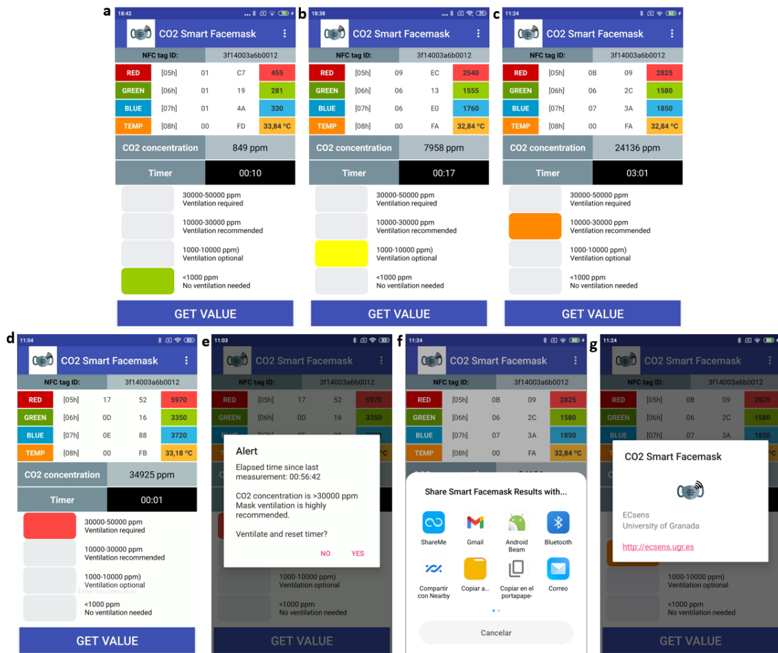
Supplementary Figure 5. a-d Screenshots of the custom-developed smartphone app showing examples of different CO 2 values and the corresponding traffic light levels as graphical indicators. e Example of dialog window showing an alarm with the elapsed time since the last measurement and the option to reset the timer. f Option “Share” where the user can send the obtained results through different messaging and/or cloud services. g “About” pop-up window containing the contact information.
