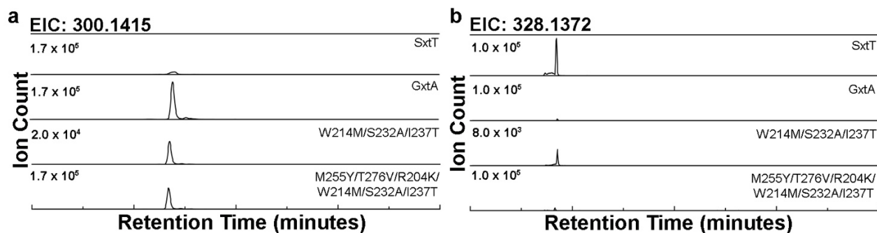
Supplementary Figure 15. A SxtT variant that combines changes in the active site, loop, and tunnel region, mirrors the selectivity of GxtA and catalyzes hydroxylation primarily at C11. (a) Extracted ion chromatograms of the SxtT, GxtA, W214M/S232A/I237T variant, and M255Y/T276V/R204K/W214M/S232A/I237T variant reaction product with of \beta -STOH. The m/z = 300.1415 value represents the mass of 11- \beta -hydroxy- \beta -STOH. (b) Extracted ion chromatograms of the SxtT, GxtA, W214M/S232A/I237T variant, and M255Y/T276V/R204K/W214M/S232A/I237T variant reaction product with \beta -STOH. The m/z = 328.1372 value represents the mass of an ethanol incorporated product. The reaction scheme for this figure can be seen in Supplementary Figure 11a.
