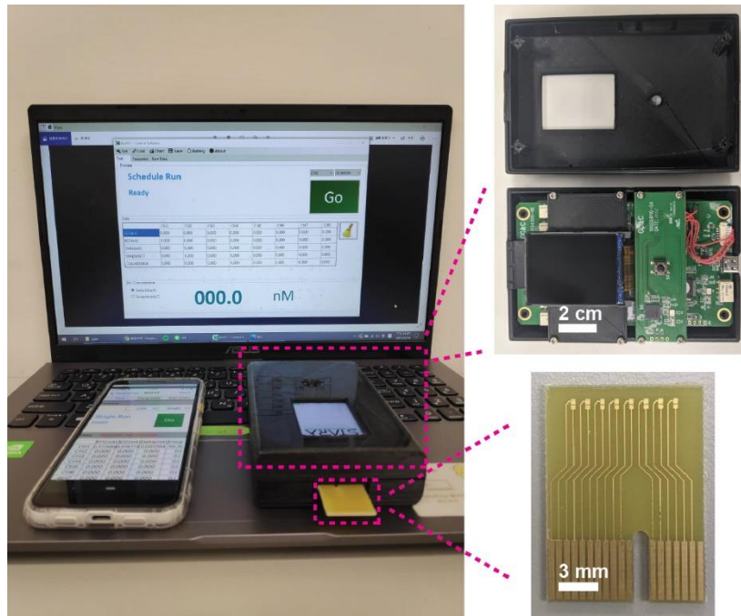
Supplemental Figure 1. Photographs of the system (left) and zoomed-in views (right) of a reader and a sensor stick. The portable testing setup shows the EDL-gated BioFET system, and measurements were recorded through a custom-written user interface as shown on a laptop screen and an iPhone.
