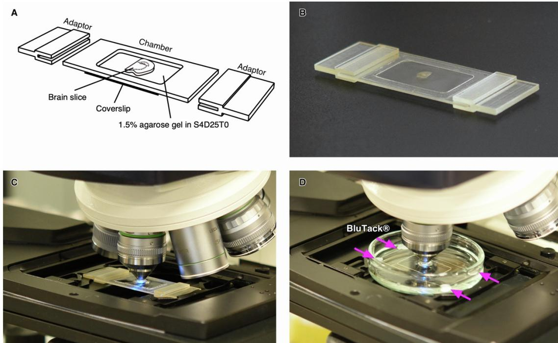
**Figure S3. Customizable 3D-printed imaging chambers for ScaleSF-treated tissues. Related to Figure 2.**
