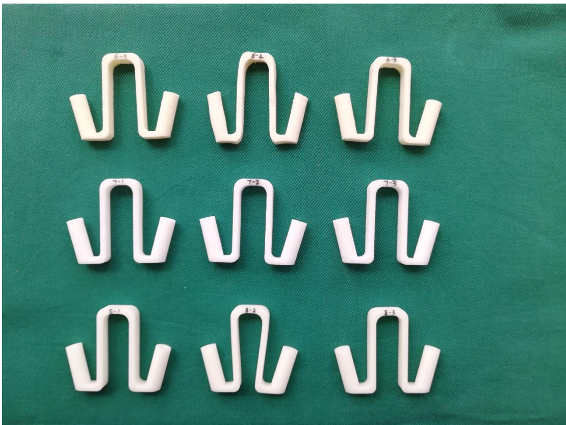
Figure S22. No deformation after EO sterilization(6-1,7-1,8-1) and plasma sterilization(6-3,7-3,8-3); Severe deformation after autoclaving(6-2, 8-2).
