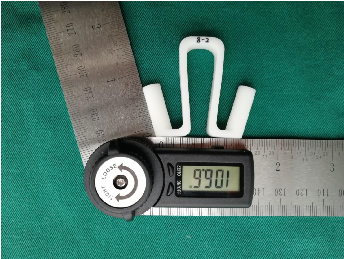
Figure S23. Obvious change in angle of guide hole.
