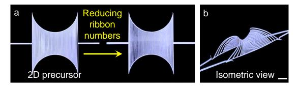
The left Fig. a shows the schematics of reducing the number of ribbons in the 2D precursor. When the number of the ribbons is reduced from 84 to 36, the morphed shape becomes frustration-free, as shown by the isometric view of the morphed shape on the right.
