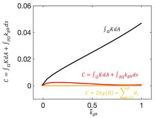
To demonstrate the variation of C from these two equations during shape shifting, we use C as a function of the normalized geodesic curvature  $\overline{k}_{gb}$  along the boundary ribbon. As shown by the figure,  $C = \int_{\Omega} K dA + \int_{\partial\Omega} k_{gb} ds$  is slightly larger than  $C = 2\pi\chi(\Omega) - \sum_{i=1}^p \theta_i$  due to the hollow spaces. However, the discrepancies between the red
