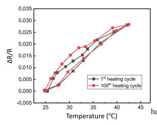
This figure shows the variation of the resistance of the heater as a function of the temperature. After 100 cycles of heating and cooling from 25°C to 42°C, the resistance-temperature curve almost does not change and the resistance is totally reversible. The maximum difference in the resistance between the two curves induced by the heating and cooling cycles is about 0.3%.
