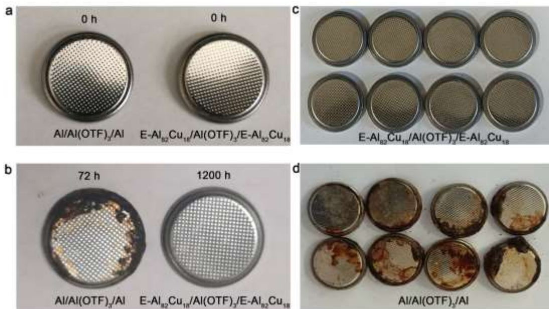
Supplementary Figure 8. Comparison of symmetric cells based on identical E-Al 82 Cu 18 and Al electrodes before and after Al stripping/plating cycles in 2 M Al(OTF) 3 aqueous electrolyte with O 2 concentration of 0.13 mg L -1 . a , Optical photograph of E-Al 82 Cu 18 (right) and Al (left) symmetric cells before Al stripping/plating cycles. b , Optical photograph of E-Al 82 Cu 18 (right) and Al (left) symmetric cells before and after Al stripping/plating cycle measurements for 1200 h and 72 h, respectively. c , d , Optical photographs for many E-Al 82 Cu 18 ( c ) and Al ( d ) symmetric cells after Al stripping/plating cycles.
