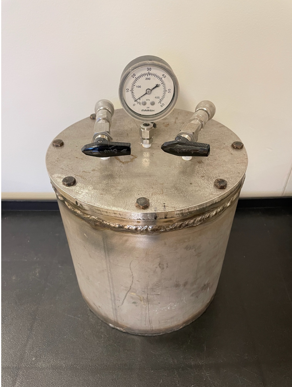
Fig. S4. Steel incubation vessel for anaerobic incubation of agar plates
