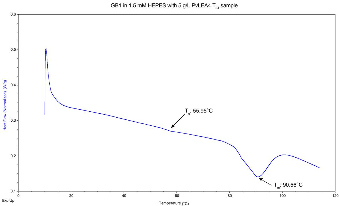
**Figure S7.** Representative differential scanning calorimetry (second scan). The glass transition- ( $T_g$ ) and denaturation- ( $T_m$ ) temperatures are indicated.
