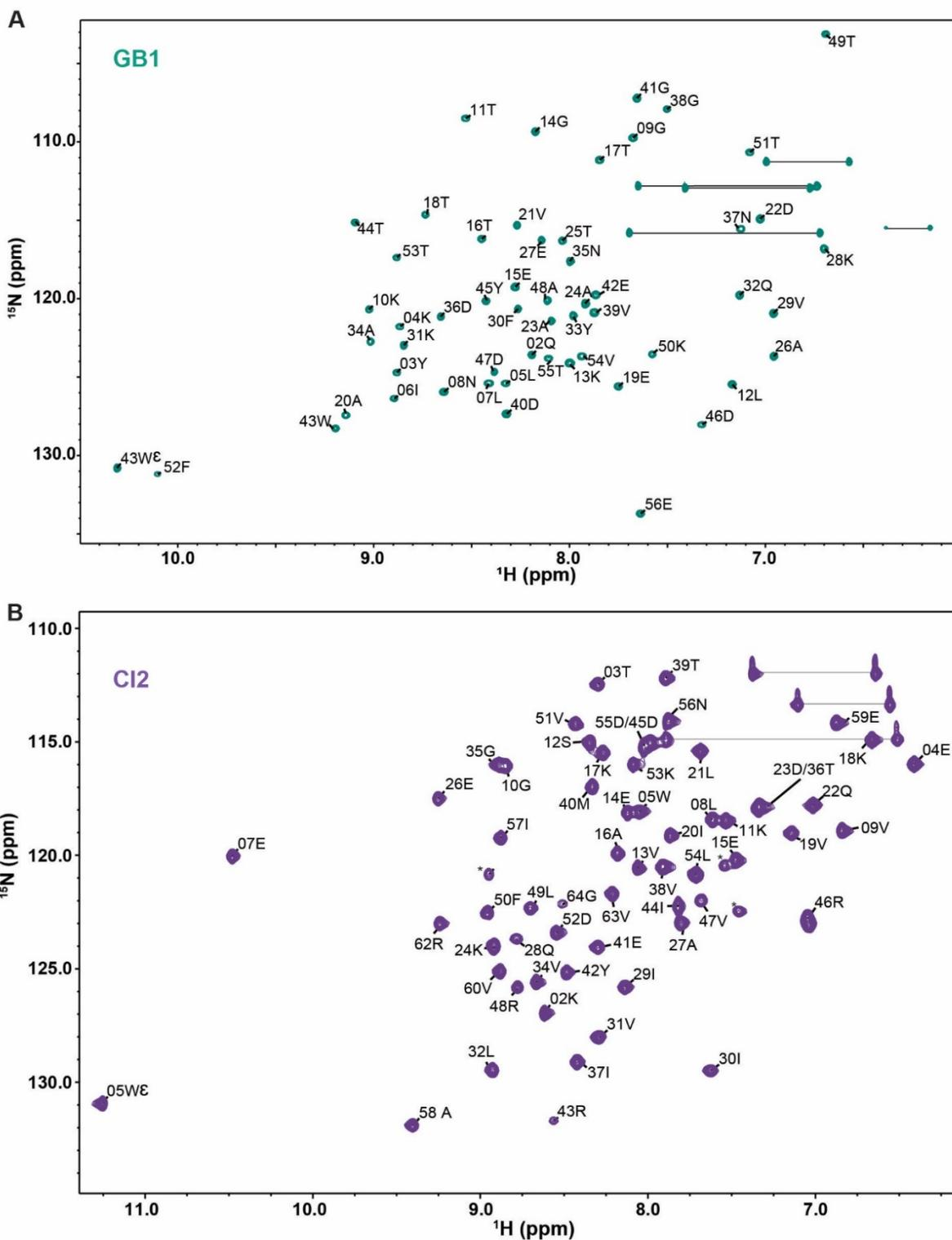
**Figure S8. Assigned  $^1\text{H}$ - $^{15}\text{N}$  HSQC spectra of client proteins under acquisition conditions for LOVE NMR. A) GB1 and B) CI2 in 100 mM citrate in 90% $\text{H}_2\text{O}$ , 10%  $\text{D}_2\text{O}$ , pH 4.5, 4°C. \*Starred resonances for CI2 probably arise from an alternative conformation.**
