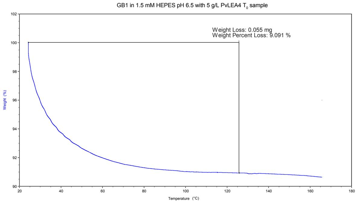
**Figure S6.** Representative data from thermogravimetric analysis. The initial change in weight due to water loss is shown.
