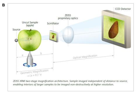
Supplemental Figure S1. X-ray computed tomography (XCT) and X-ray microscopy (XRM)
