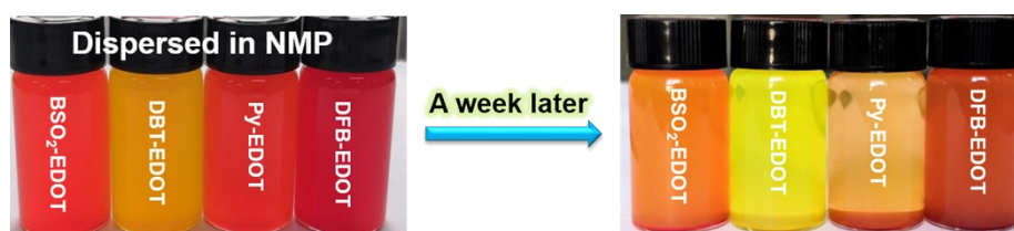
Fig. S2 Photograph of CPs dispersed in NMP via conventional sonication for 30 min, and then standing for a week.
