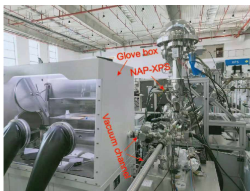
Supplementary Figure 27. The display of quasi in situ alkaline HER setup. Photo of the vacuum-connected glove box and NAP-XPS system, where the vacuum connection of glove box and NAP-XPS setup is achieved by vacuum channels, and the electrochemically treated sample can be transferred to the analysis chamber of NAP-XPS without air interference.
