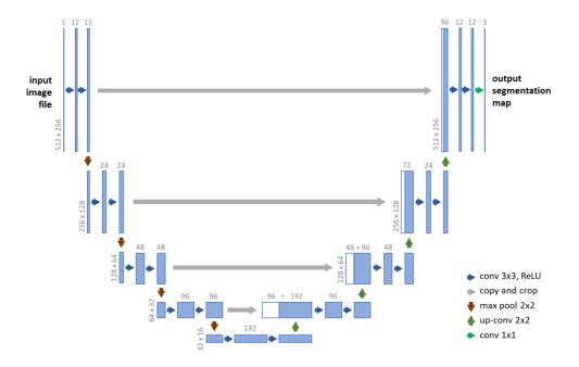
Supplementary Figure 1. Modified U-net architecture used for AS-OCT image segmentation.
