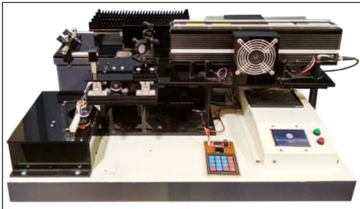
Figure S2: In-house built CO 2 laser based fiber optic bending machine
