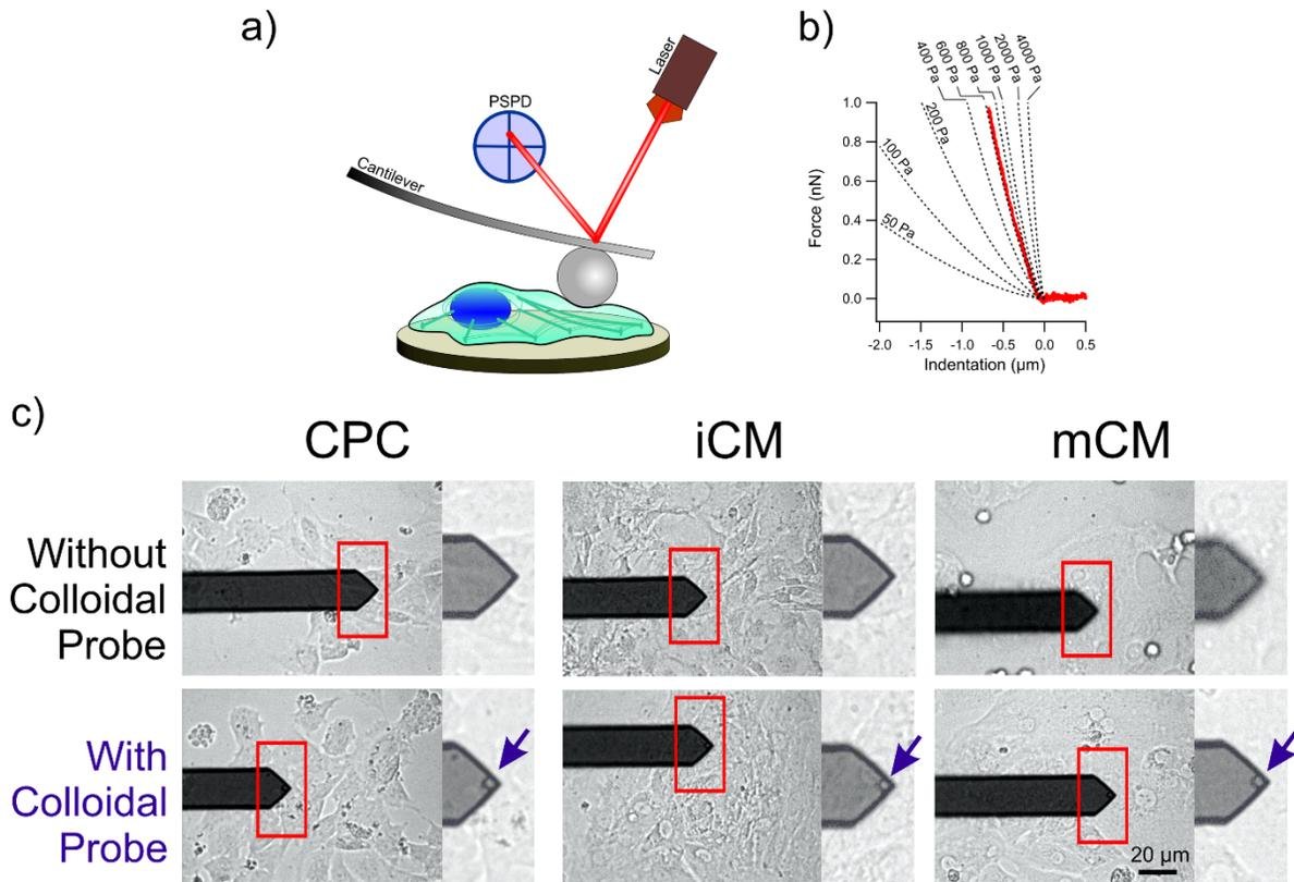
**Supplemental Figure 5: AFM colloidal force spectroscopy indentation experiments.**
