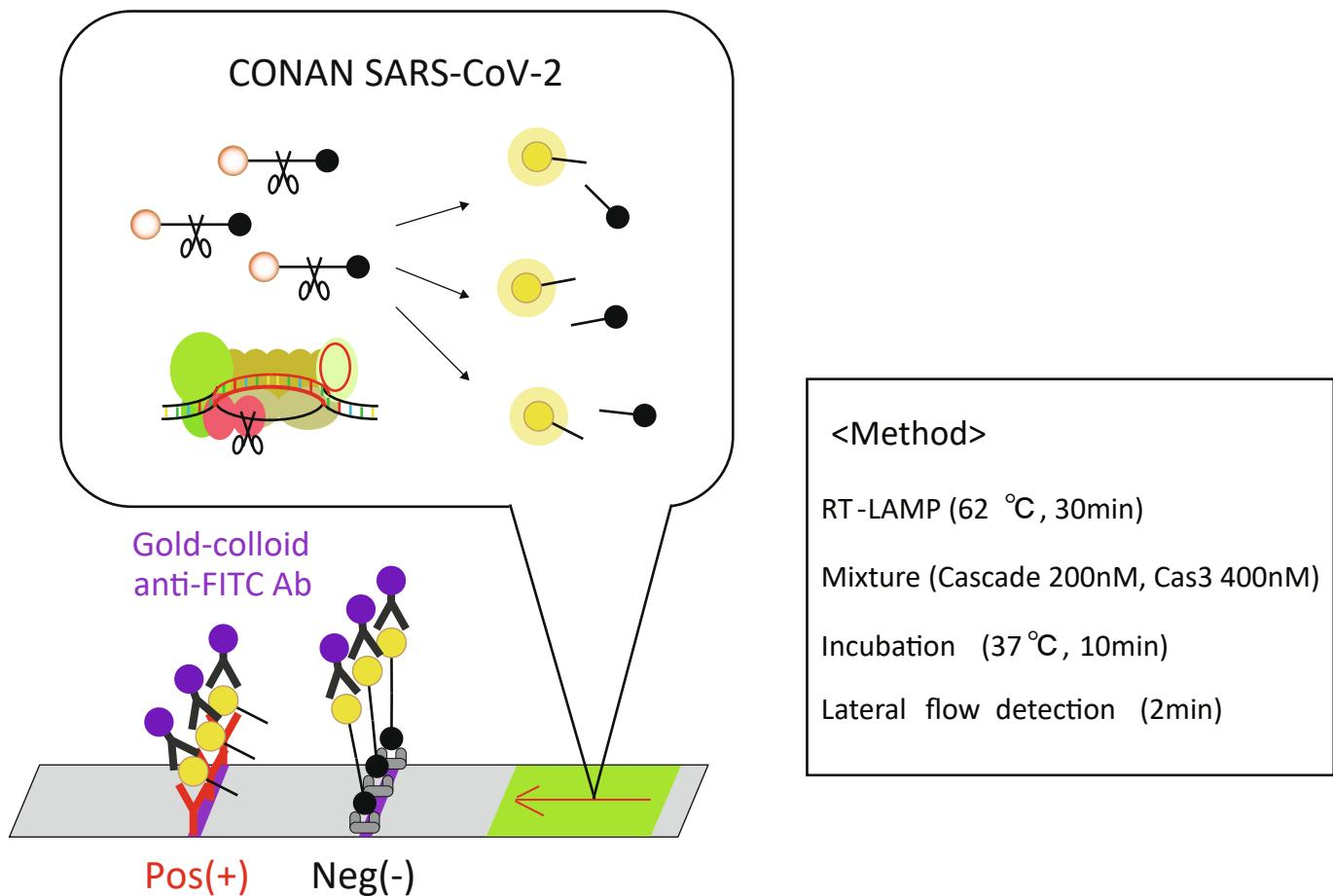
**Fig. S8. Lateral-flow detection with CONAN. Related to Fig. 2d and STAR Methods.** Abundant uncleaved FQ-labeled ssDNA reporter accumulates anti-FAM antibody-gold nanoparticle conjugates at the first line (negative) on the strip, while cleaved reporter reduce accumulation at the first line and result in signal on the second line (positive) for <2 min flow.
