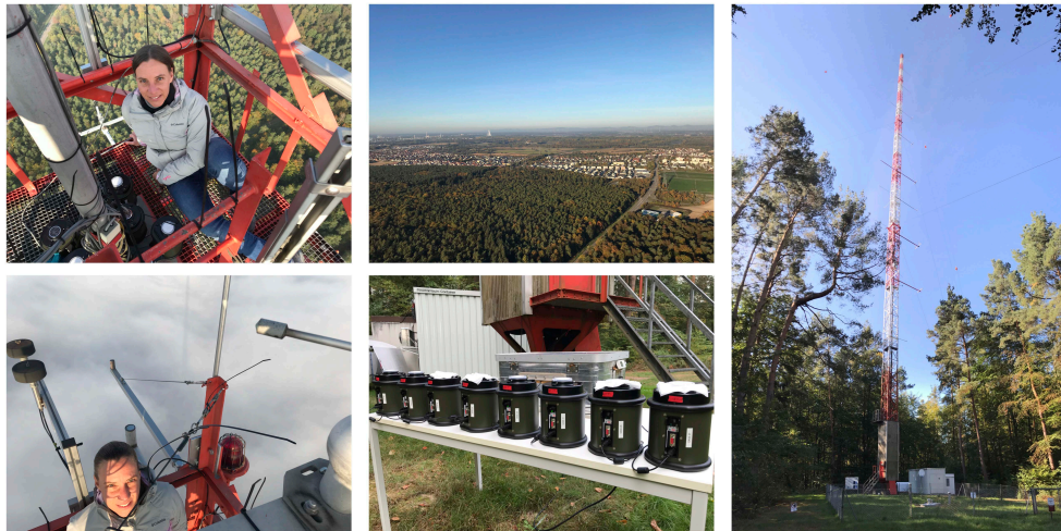
Figure S17. Temporal and vertical distribution of airborne microbial organisms in the near-surface atmosphere. Experimental set-up. SASS air samplers were placed on the uppermost platform of the tower (200m), as well as near the base of the tower (~0.75m). Air samples were collected at the top and bottom for 5 consecutive days, in 4-hour increments, and a sampling duration of 2 hours. For each time point, samples were collected in duplicates.
