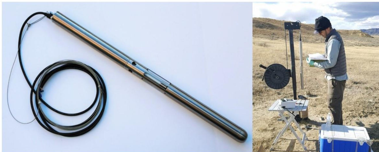
Supplementary Figure 1.) Photographs of the Subsurface Environmental Sampler (SES) (image on right, courtesy of Jesse Barnhart) used to obtain coal associated communities. The authors affirm that the individual imaged in the right provided informed consent for publication of the image.
