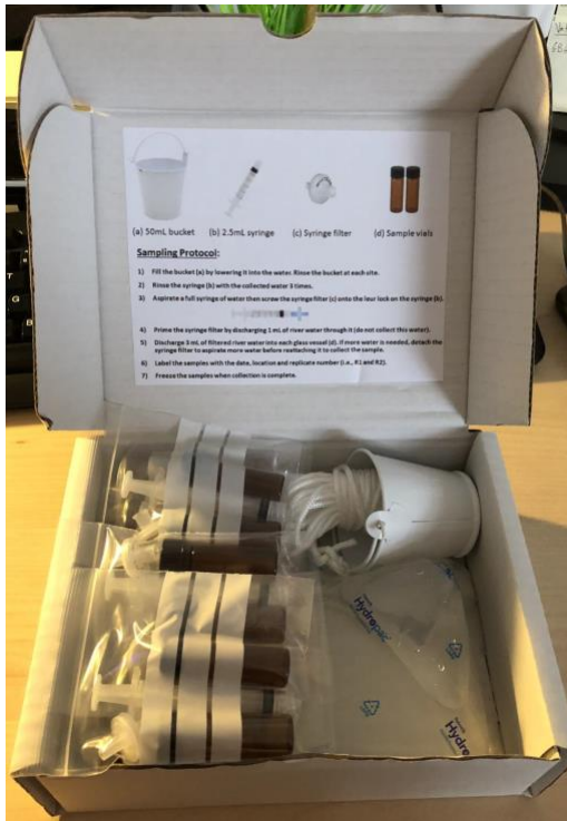
Image S1. Miniaturised sampling kit used for all sampling campaigns in this global study (1)
