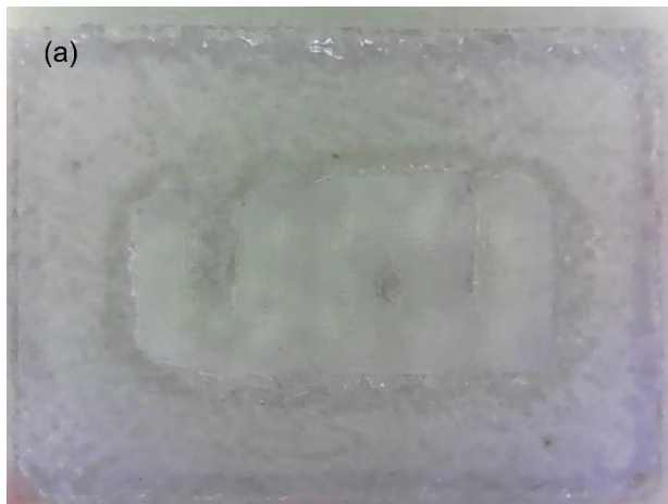
Supplementary Figure S10. Optical imaging of designed resin structure clean (b) and embedded in silicone lubricant (a).
