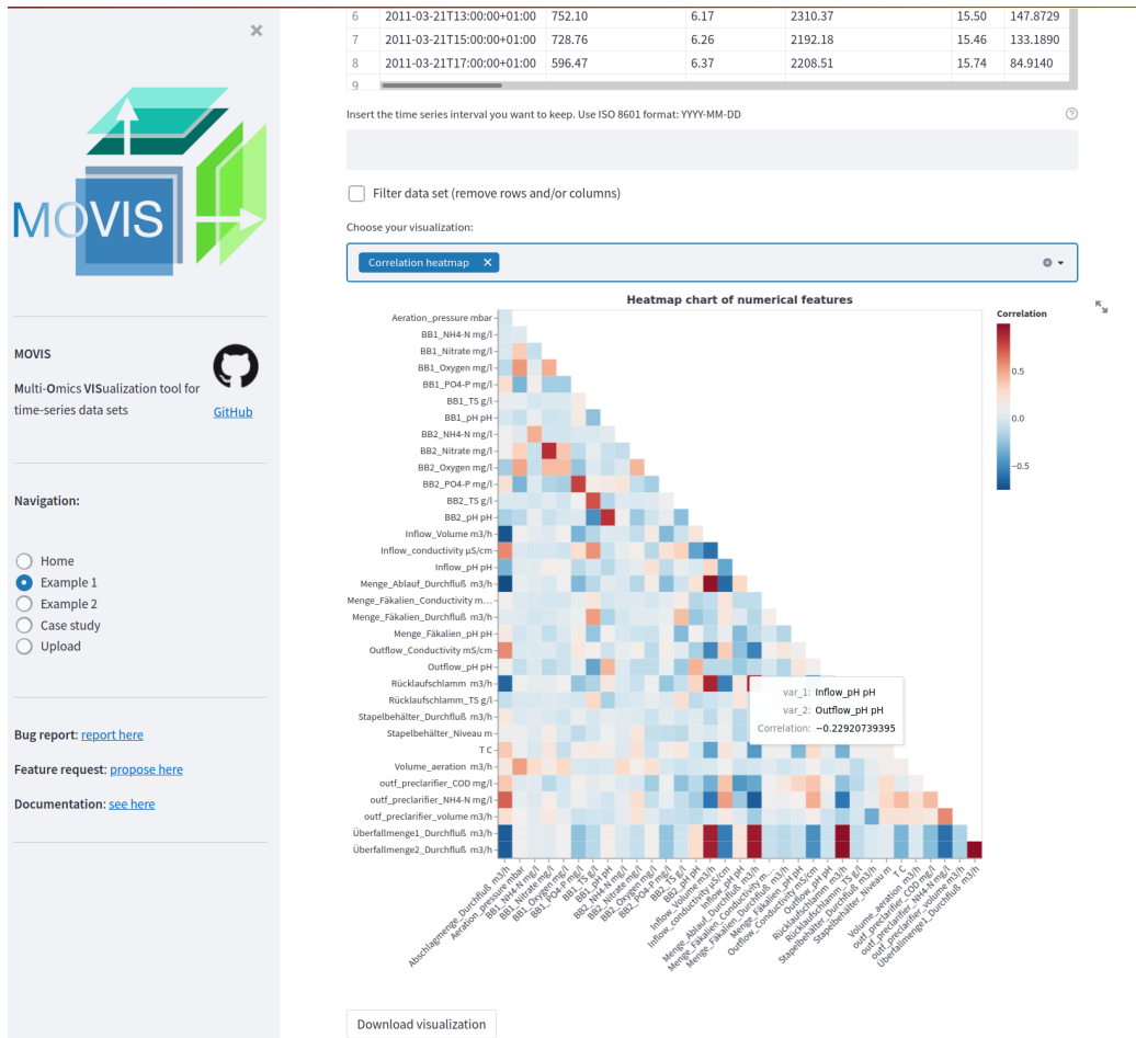
Figure 7: Triangular heatmap of all features in the physico-chemical properties data set. A diverging color scheme palette is selected to showcase low and high correlations with less emphasis on the mid-range values. A tooltip is available to investigate specific heatmap cells.
