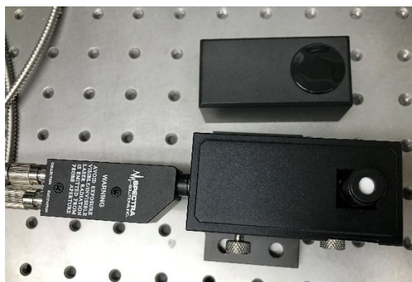
Figure S1. General-purpose Raman probe and probe/cuvette holder made by Spectra solutions Inc.
