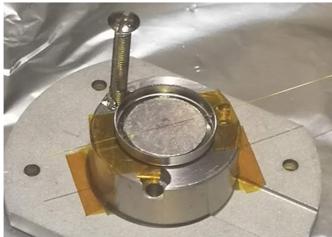
Supplementary Figure 13 | Photographs of a real FBG sensor at the anode/solid electrolyte interface.
