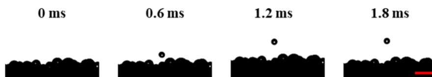
Figure S12. Coalescence-induced condensate droplet jumping on a Cu superhydrophobic surface. Scale bar: 1 mm.
