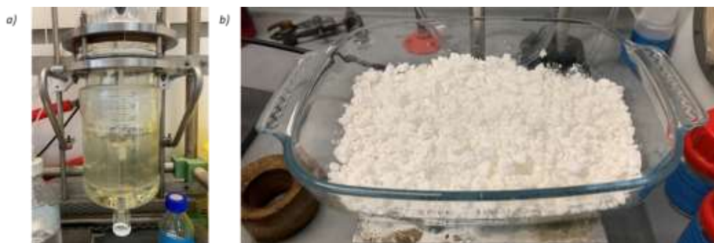
Figure S8: a) A 1 L scale biotransformation was carried out in a 2L Mettler Toledo AP01 jacketed vessel cooled to 4°C. b) N -Hydroxy-cytidine 4 crystallized in situ to give 137 g of a white solid in 71% isolated yield and >95% purity following filtration, washing and drying.
