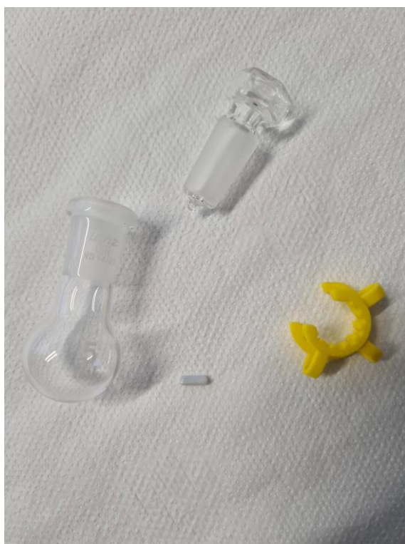
Supporting Photo S10. 5 mL round-bottomed flask, stirring bar, ground glass joint with plastic clamp.
