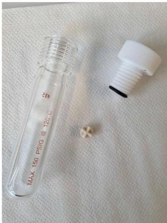
Supporting Photo S2. 21 mL ACE pressure tube, magnetic stirrer and screw cap.
