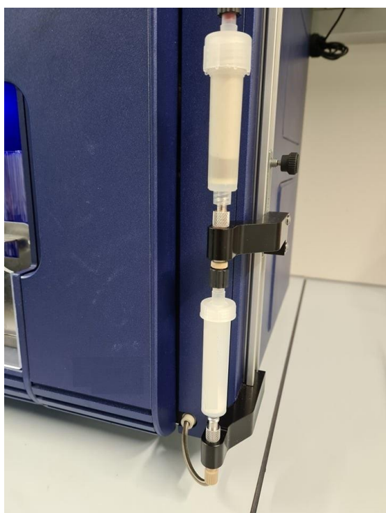
Supporting Photo S15. Purification with dryload silica column chromatography using Interchim puriFlash ® XS520.
