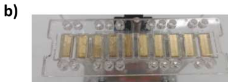
Figure S3. a) The permanent magnet (PM) actuation system. The micro servo motor and the pull up system are visible on the right. b) The ten permanent magnets in contact with the bottom part of the microfluidic chip.
