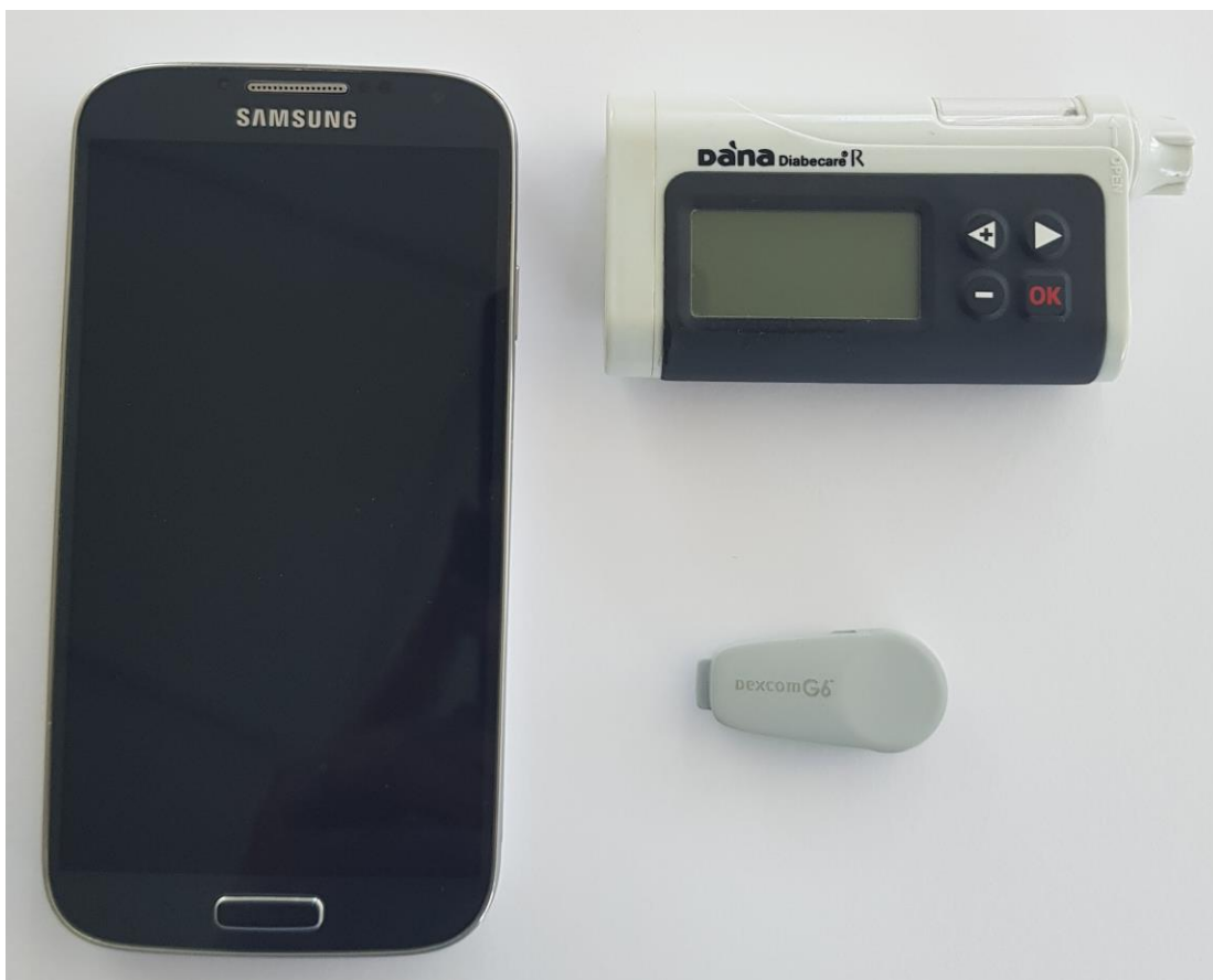
Figure 1. CamAPS FX comprises Samsung Galaxy phone (or similar) running Cambridge control algorithm, Dana insulin pump (Sooil), G6 real-time CGM sensor (Dexcom).
