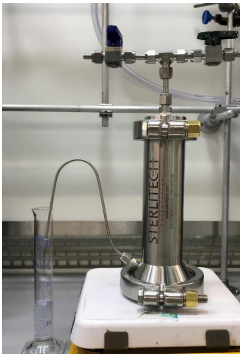
Figure S22. To evaluate the separation performance of the CC3-PAN membranes, the permeance and selectivity measurements were carried out using a commercial bench-scale dead-end stirred-cell filtration unit (Sterlitech® HP4750 stirred cell) that was kept under 10 bar upstream nitrogen pressure at room temperature. The agitation speed was kept at 400 rpm during the measurements. The membrane was cut into a coupon with a diameter of 4.7 cm to fix at the bottom of the cell.
