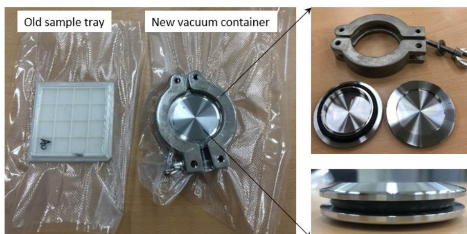
Figure R1. Previous low-vacuum package with sample tray and the newly-developed
