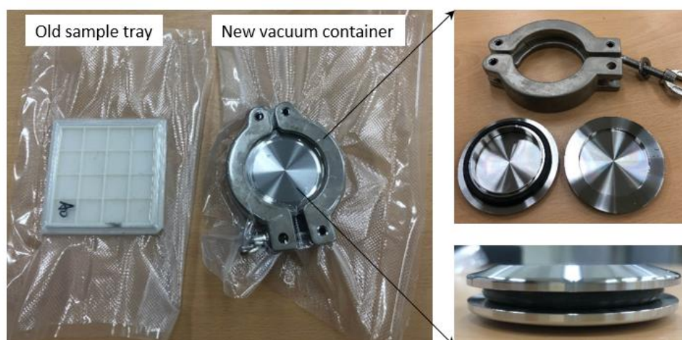
Figure R1. Previous low-vacuum package with sample tray and the newly-developed high-vacuum metal/rubber/metal container. The new container can be first high-vacuumed under an inert atmosphere using the anti-chamber in an \text{N}_2 -filled glove box, then vacuumed
