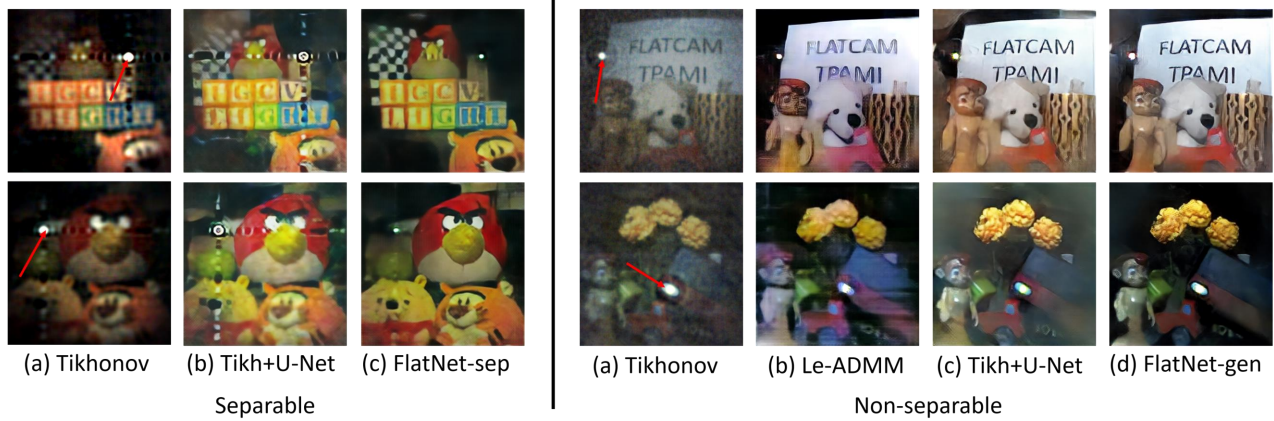
Fig. 11. Reconstruction of scenes with bright objects (LED) using FlatCam and PhlatCam. Artifacts occurring in Tikhonov reconstructions are amplified by Tikh+U-Net reconstruction. While Le-ADMM performs slightly better than Tikh+U-Net for PhlatCam, it is outperformed by FlatNet-gen
