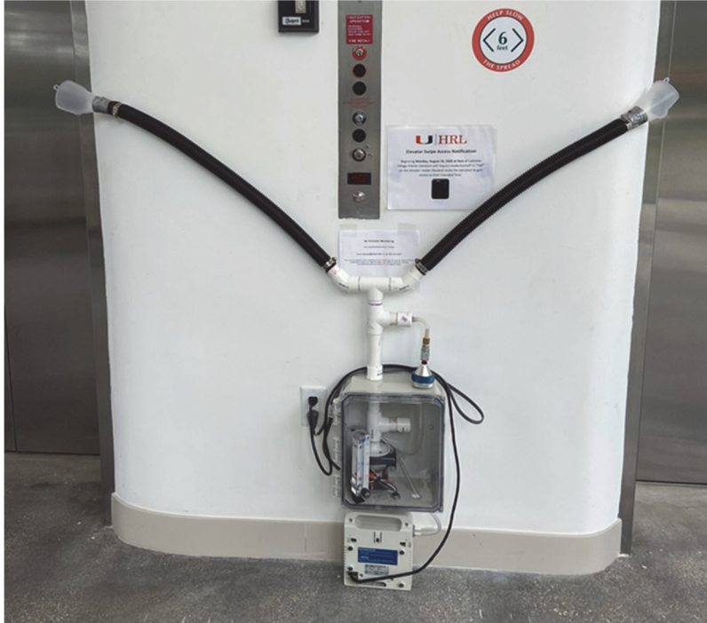
Figure S2: Active air sampling setup in lobby of Lakeside Village. Sterile 47mm polycarbonate membrane filters with a pore size of 0.4 \mu\text{m} were used in our customized impactors, connected with a vacuum pump that ran in 25h increments at a flow rate of 10-12 l/minute to collect particles and aerosols within the lobby.
