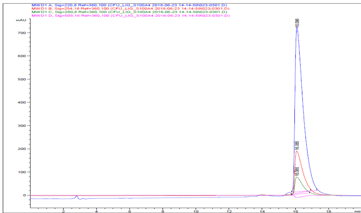
Figure S25. The MS spectra and the HPLC chromatogram of fTM (Column: Phenomenex Luna C18 (250 x 4.6 mm, particle size: 5 micron, pore size: 100 Å); Gradient: 30-50% 20min 1.2 mL min -1 )
