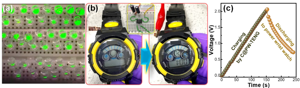
Figure S6. (a) Commercial LEDs connected in series and (b) wristwatch display powered either directly by the C@PW-TENG or through a rectifier followed by a capacitor. (c) The charging and discharging curve of the commercial capacitor connected in between the C@PW-TENG and wristwatch through a rectifier.
