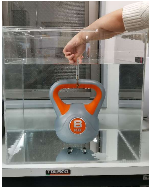
Supplementary Fig. 42 | A bonded aluminum rod raises 8-kg.
