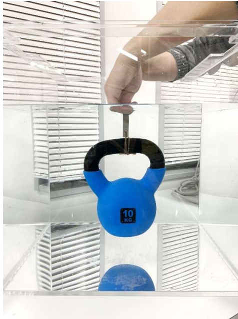
Supplementary Fig. 10 | Steel adhered with P(5HS 11% - co -S 89% ) can lift 10-kg.
