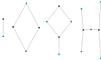
Figure S 2: Possible occurrences of poor matches in four multiple-match clusters, or connected components (CCs), with reference features in dark blue, target features in light blue). From left to right: single match; multiple-match cluster with two features in both reference and target; multiple-match cluster with two features in reference and three in target; multiple-match cluster with two reference and five target features. The single match cluster will yield one match, while all others may each yield (in this example) a maximum of two matches per cluster.
