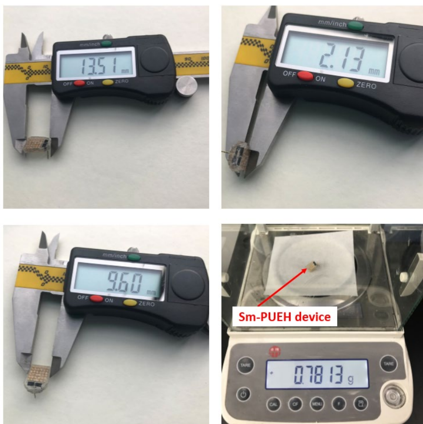
Fig. S6. Size and mass measurement for Sm-PUEH device.
